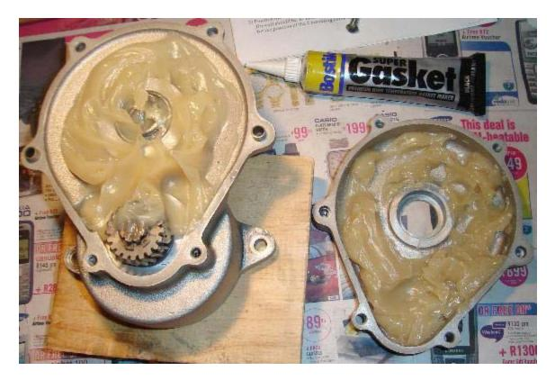
15) A thin bead of sealant has been applied to the mating surfaces and the two halves are brought together. If your prop-shaft output bearing was subject to spinning in it's housing, apply thread-locker compound around the seat area first.
