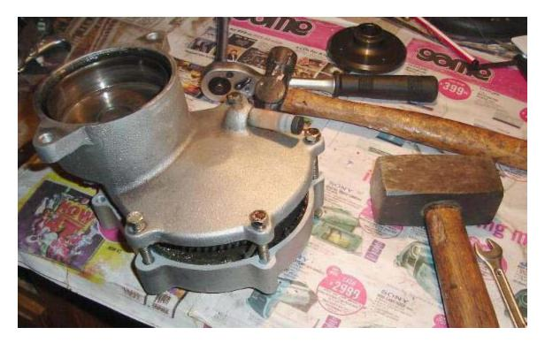
6) Here, the bolts have been tapped through to their maximum extent and can be removed. The old grease can be seen, still fairly clean, to be expected on a low hours box. Looks like a blue silicone based sealant was used previously see the stringy bit still clinging on between each half of the case. It did the job; I had no leaks along the join.
