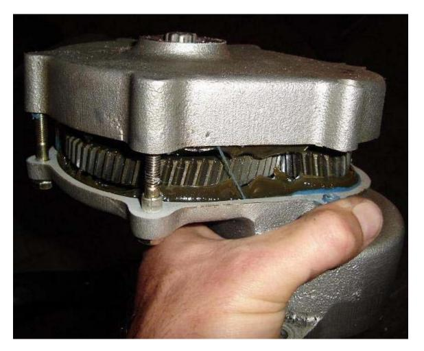
7) Using two large screwdrivers as levers, the main gear can be levered out. Be careful not to damage the mating surfaces with the screwdrivers. It should pop out fairly easily. If not, make sure that the force is applied evenly to each side and use pieces of wood to lever against to protect the case.
