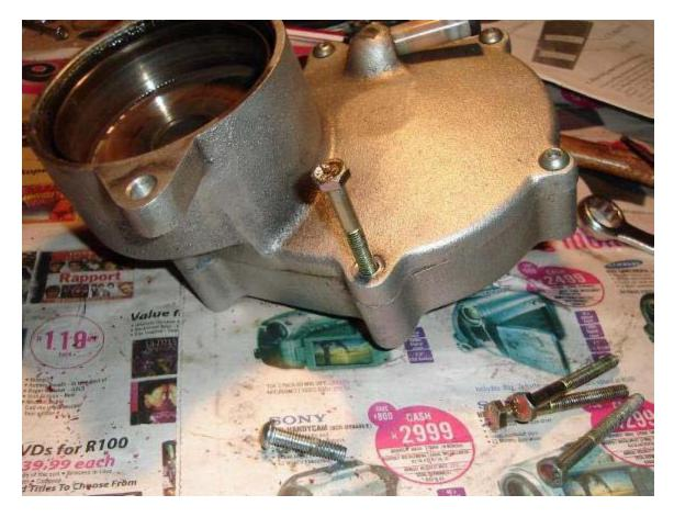
5) The four bolts in place, screwed in as far as possible for maximum thread contact. Don't force them in too far and strip the threads though. Supporting the box by the clutch (i.e. Suspending the lower part of the box in the air) tap down successively on each of the four bolts gently to break the seal and separate the case. This should pop apart fairly easily once the seal is broken.
