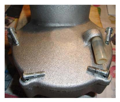
17) Refit the box and drift on the prop hub, making sure the shaft and hub contact surfaces are spotless. There should be no rocking and the shaft should sit in 1-2mm as shown in the picture below to allow the retaining bolt to draw down. Apply a little thread-locking compound to the screw and tighten up, using 2-3 thick washers. Be careful not to bottom the screw if it's too long.
