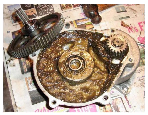
9) Scribe a line along the top of the clutch bell against the casing. This will indicate how far the bell/shaft needs to be driven in on reassembly. Note the small groove in the lower casing flange to let the excess grease ooze out. It will be an easy inspection point to monitor the new bearing's grease retention in future too.
