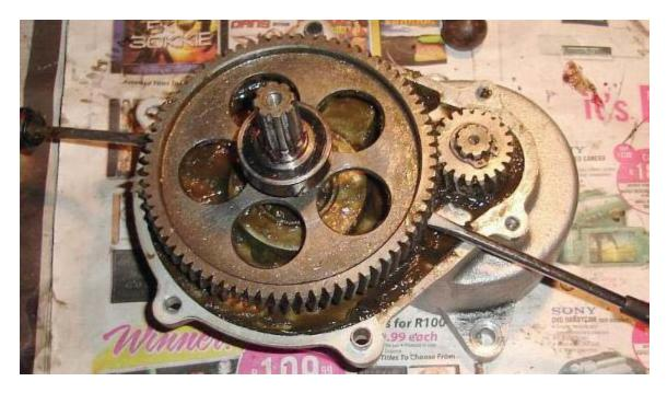
8) The fun part, cleaning out all the old grease! Remove the circlip from the small pinion so long.
