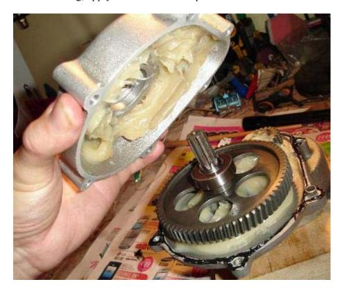
16) Note that the two shorter screws are closer in the picture below. Note the missing black vent cap cover, it melted in the oven, oops!! (I have since procured a toothpaste cap drilled 1.5mm in the centre, hot glued on, which is working admirably so far).
