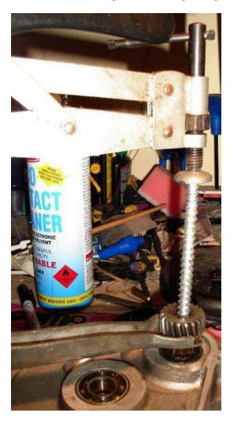
12) Just look at that cool frosty finish on the main gear, makes me want to reach into the fridge for a cool one.... The gear spent an hour or so in the freezer to cool it down. I then warmed the bearing with a mini blowtorch to maximize the temperature differential (and therefore clearance) prior to pulling the bearing off. It was quite tight. I don't think you would be able to lever this one off without the correct tool. Drive a new bearing on
