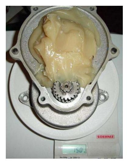
14) Probably unnecessary, but I distributed the grease between the two halves. Don't get it in the bearing seat (right side cover) or it could promote bearing spin in the housing. See the brand of sealant I used in the picture below, it's a black silicone based sealant.
