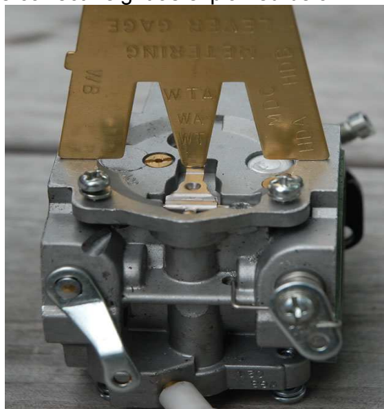
Setting the Metering Lever height. Photo by Richard Cobb.
