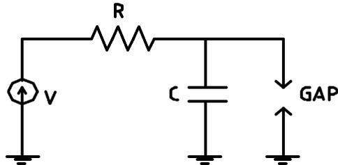
**Figure 2.** A self-oscillating circuit.
