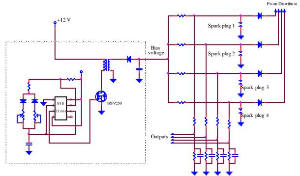
**Figure 5.** The four-channel measurement circuit, including the high voltage source.
