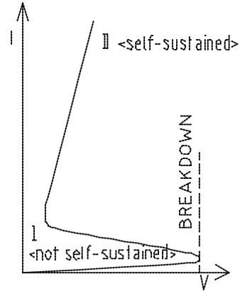
**Figure 3.** A simplified volt-ampere characteristic of a discharge gap.
