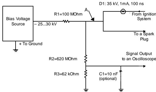
**Figure 1.** Schematic diagram of the measurement circuit. An additional diode can be installed in the line marked "A"
