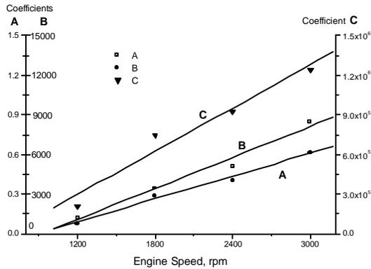
**Figure 10.** The polynomial coefficients are linear functions of engine speed.
