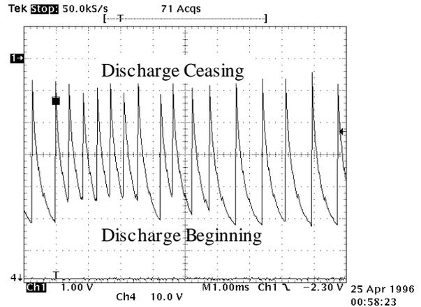
**Figure 4.** A sample waveform of the oscillations in the measurement circuit.
