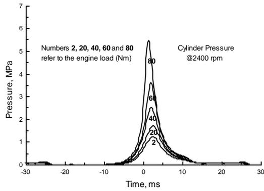
**Figure 7.** Cylinder pressure at 2400 rpm, different loads.
