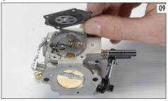
⚠ATTENTION: The carburettor is made of many small and fragile parts. Be very careful during all the phases with particular attention to the idling and its springs; they both must not be touched.
