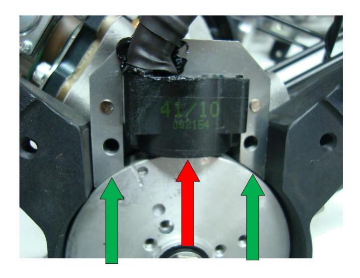
The gap between coil SELETTRA and flywheel SELETTRA must be 0,30 mm in the central part (red indicator) and 0,30 mm in the lateral parts (green indicators).
