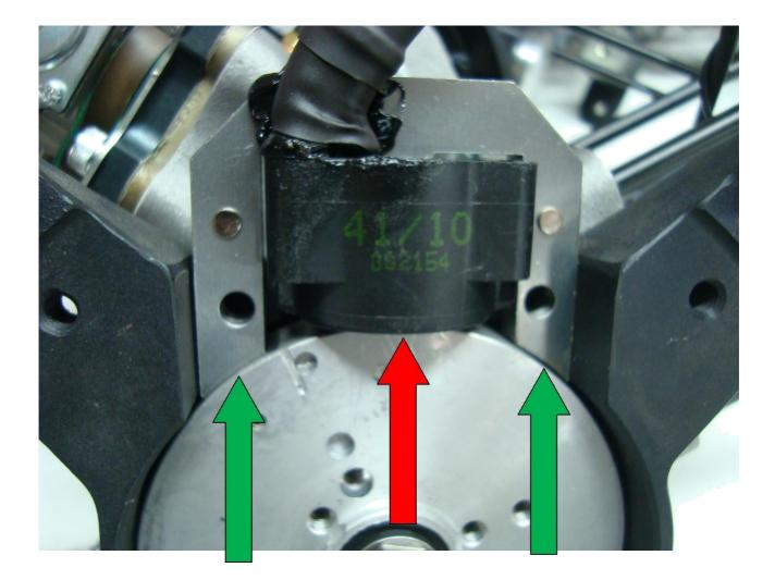
The gap between coil IDM and flywheel IDM must be 0,35 mm in the central part (red indicator) and 0,50 mm in the lateral parts (green indicators).
