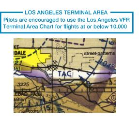
Inset coverage is shown on appropriate Sectionals by a 1/8" masked line as indicated below. A note to this effect appears near the masked boundary line.
