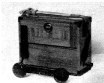
Fig. 7, 8 and 9 Field telephone from Elektrisk Bureau, Oslo above, closed for transport middle, open for use below, lid shut for use in bad weather
