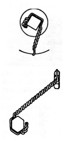
These units are used where a nut or bolt does not have a hole for safety wire. You install them under the nut/bolt bend the tabs over the side of the nut/bolt and then safety wire the tab with the hole in it.
