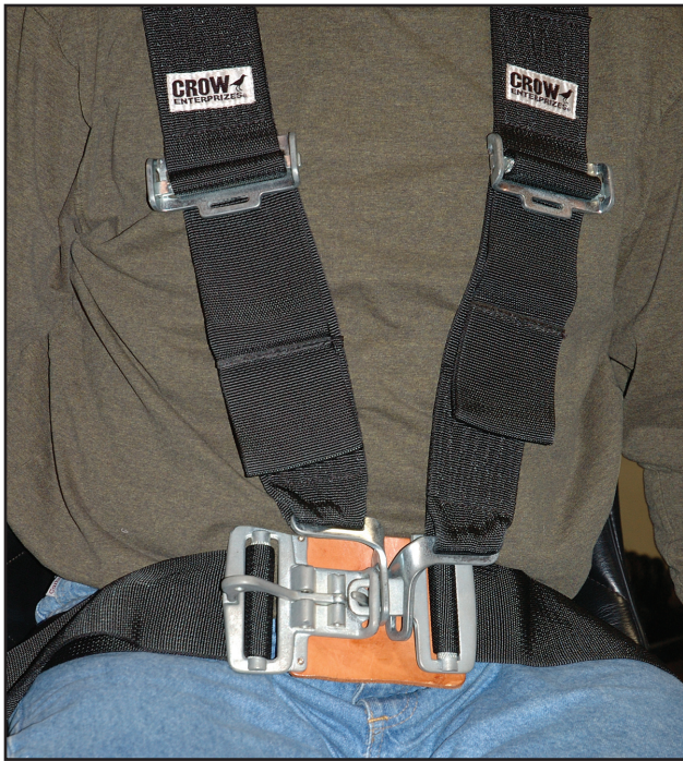
Figure 3-3. The harness should be fastened snug but not tight.
