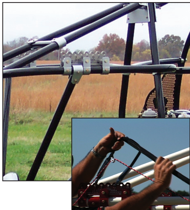
Figure 3-4. Multiple attachment points for the wing as a means to adjust the wing hang point.
