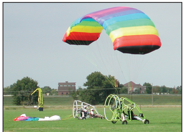
Figure 7-3. Pressurizing, or kiting, the wing.
