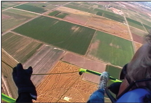
Figure 6-6. Push the foot control and pull the steering line smoothly and slowly.
