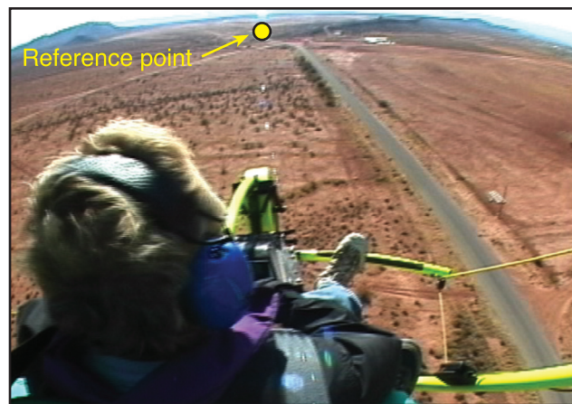
Figure 6-4. Nose reference for straight-and-level flight.
