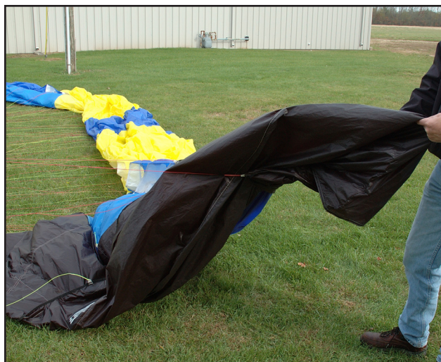
Figure 5-21. A simulated line-over.
