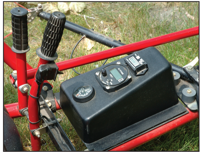
Figure 3-6. Some instrument panels will have just a few digital or analog gauges for EGT and RPM.
