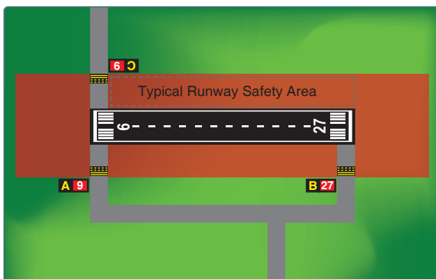
Figure 14-7. Runway Safety Area.
