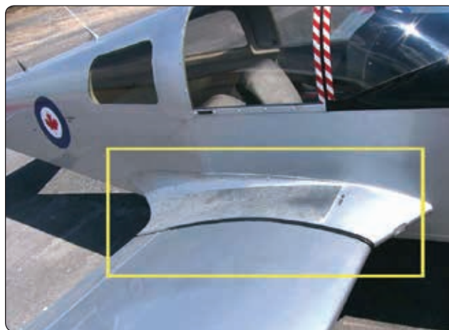
Figure 5-8. A wing root can cause interference drag.
