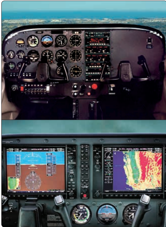
Figure 3-18. Analog display (top) and digital display (bottom) from a Cessna 172.
