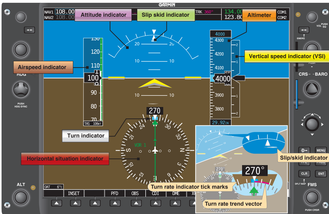
Figure 8-12. Primary flight display (PFD). Note that the actual location of indications vary depending on manufacturers.
