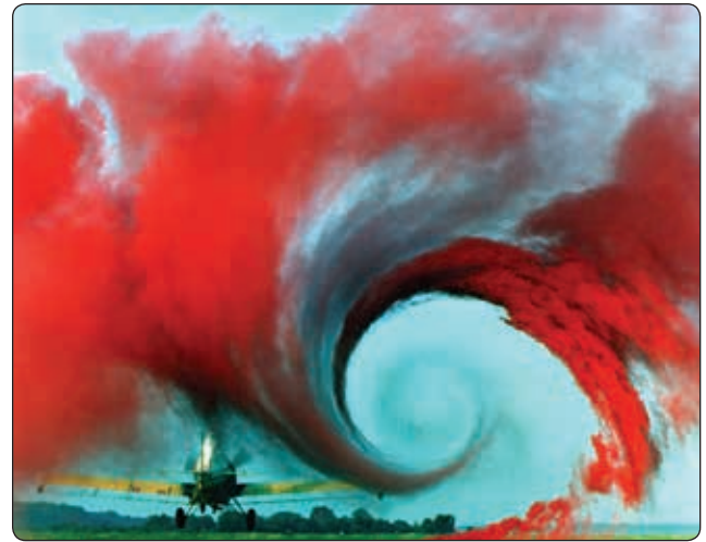
Figure 5-9. Wingtip vortex from a crop duster.
