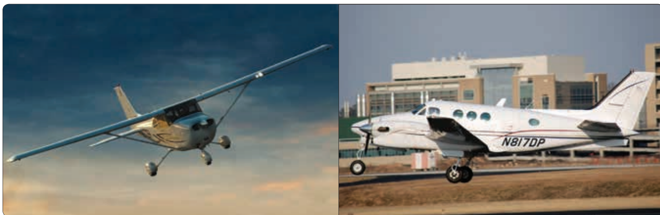
Figure 7-39. Fixed (left) and retractable (right) gear airplanes.
