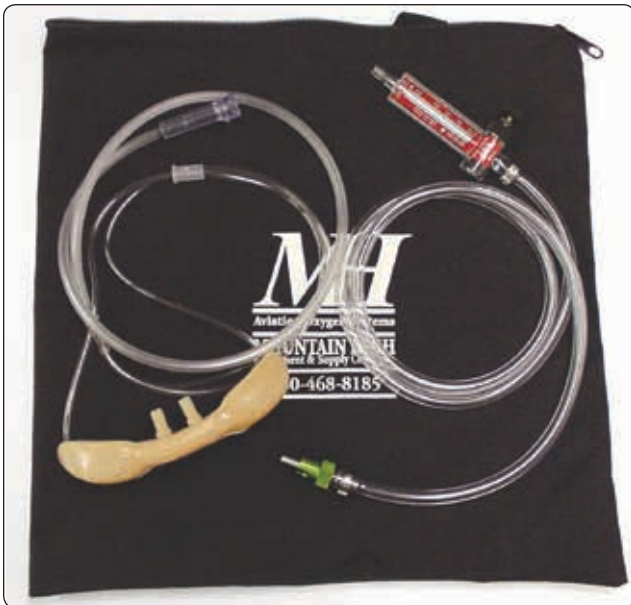
Figure 7-44. Cannula with green flow detector.
