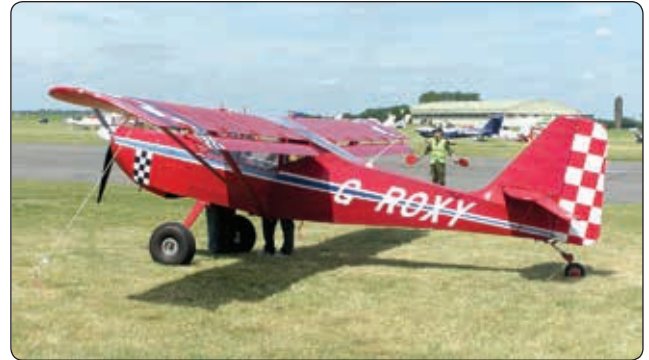
Figure 6-9. Flaperons on a Skystar Kitfox MK 7.
